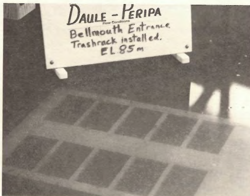
Figure 61.—No vortex formed at reservoir EL 85, Q = 250 \text{ m}^3/\text{s} , with the trashrack. P801-D-79614.
