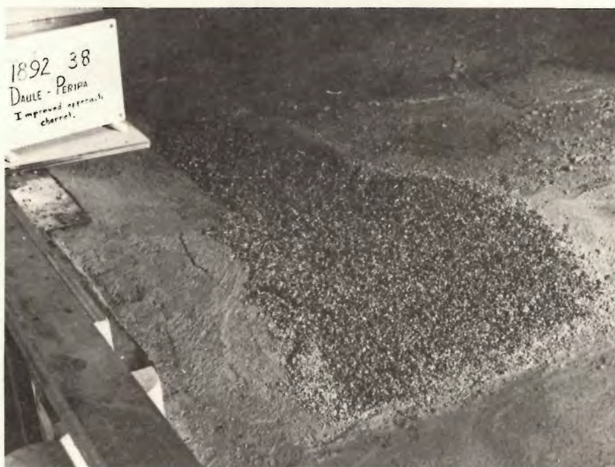
Figure 8.—Right side of approach channel adjacent to crest, with original topography restored. P801-D-79580.
