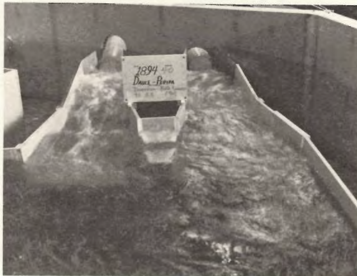
Figure 43.—Diversion stilling basin operation, reservoir EL 53, Q = 2007.9 \text{ m}^3/\text{s} , tailwater EL 33.6. P801-D-79601.
