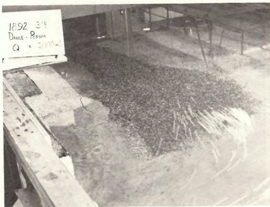
Figure 9.—Flow pattern adjacent to crest: Q = 2000 \text{ m}^3/\text{s} for the improved channel. P801-D-79581.
