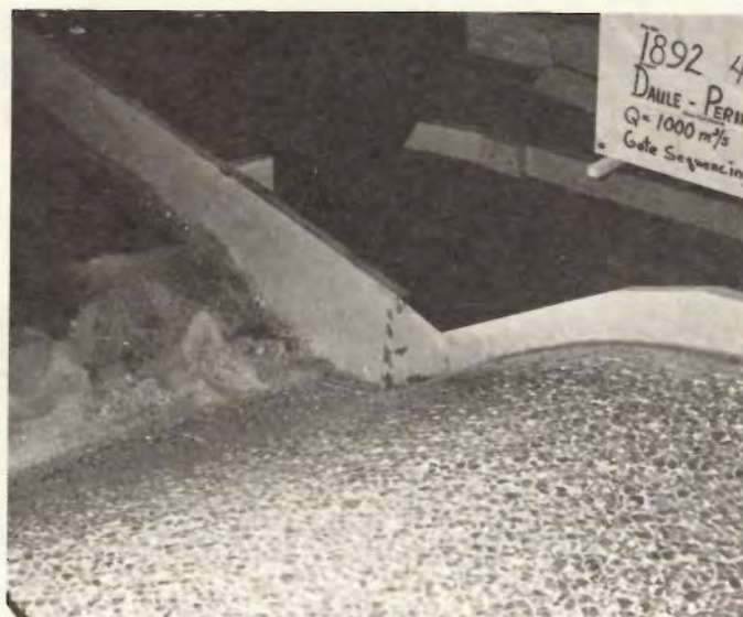
Figure 23.—Spillway stilling basin operation for Q = 1000 \text{ m}^3/\text{s} and tailwater EL 25. P801-D-79588.
