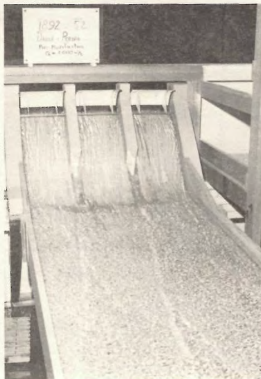
Figure 12.—Piers streamlined and shortened to STA 1 + 20.5. P801-D-79584.
