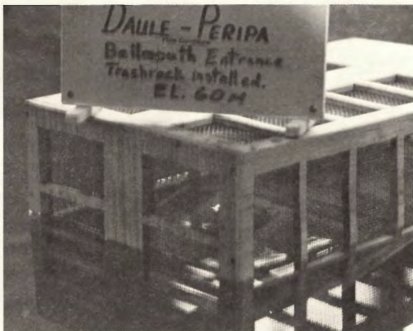
Figure 59.—No vortex formed at reservoir EL 60, Q = 100 \text{ m}^3/\text{s} , with the trashrack. P801-D-79612.
