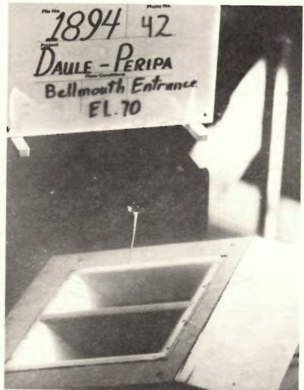
Figure 55.—Vortex at the bellmouth intake for reservoir EL 70 without the trashrack. P801-D-79608.
