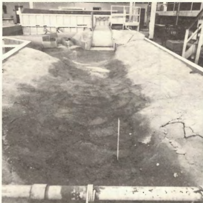
Figure 27.—Stabilized riverbed for spillway model. P801-D-79591.
