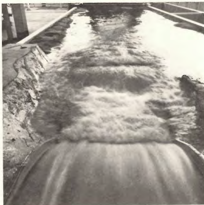
Figure 25.—Spillway stilling basin operation for Q = 3600 \text{ m}^3/\text{s} and tailwater EL 41.5. P801-D-79590.
