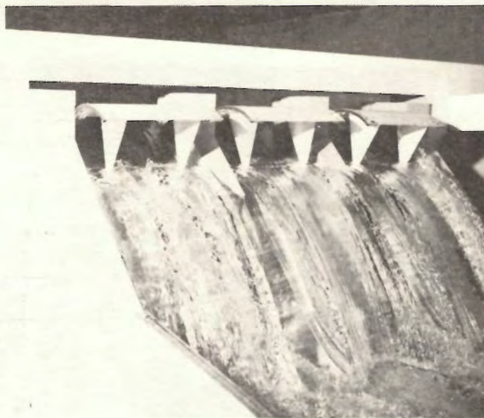
Figure 11.—Submergence of all trunnions: Q = 3600 \text{ m}^3/\text{s} . P801-D-79583.
