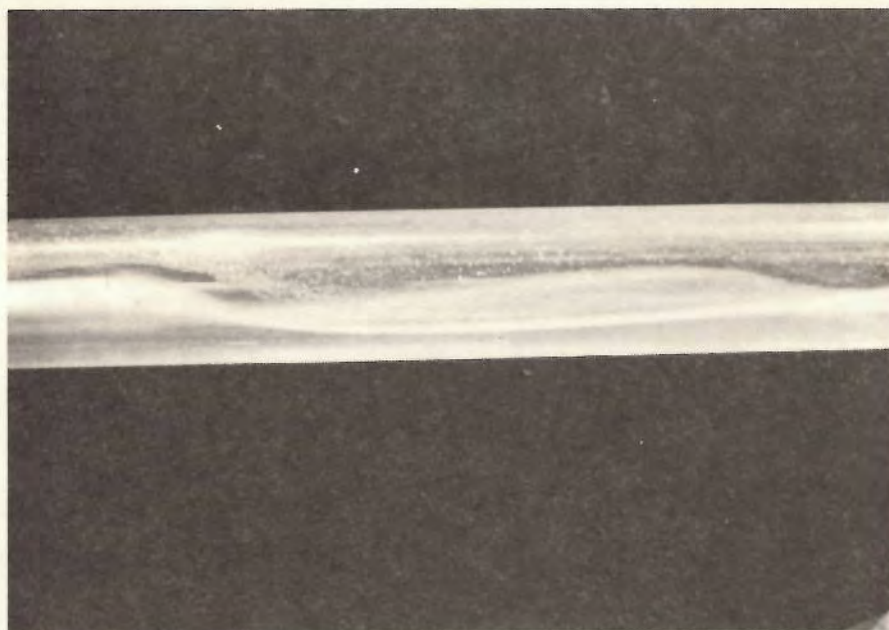
Figure 47.—Oscillating flow downstream of the tunnel bend with reservoir EL 85, Q = 422 \text{ m}^3/\text{s} . P801-D-79604.
