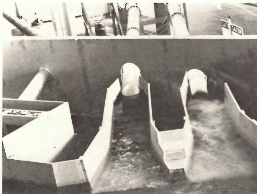
Figure 48.—Stilling basin operation for Q = 422 \text{ m}^3/\text{s} and reservoir EL 85. P801-D-79605.
